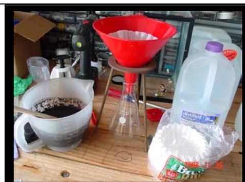
The solution is hot-filtered to remove the insoluble material, and the filtrate received into a flask
