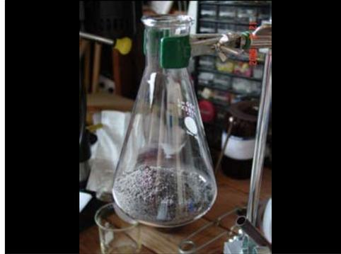
The ash is added to a flask and mixed with distilled water
