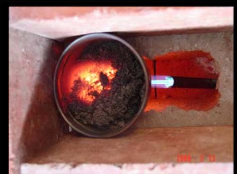
The material is further reduced in a crucible to burn off most of the remaining carbon and carbon compounds
