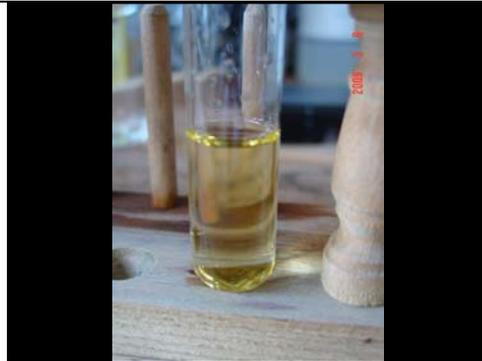
A small portion of the solution is added to a test tube and sulfuric acid is added to decrease the pH. Hydrogen peroxide is added to liberate some of the iodine as an element. Note the pale yellow color. Is this iodine?
